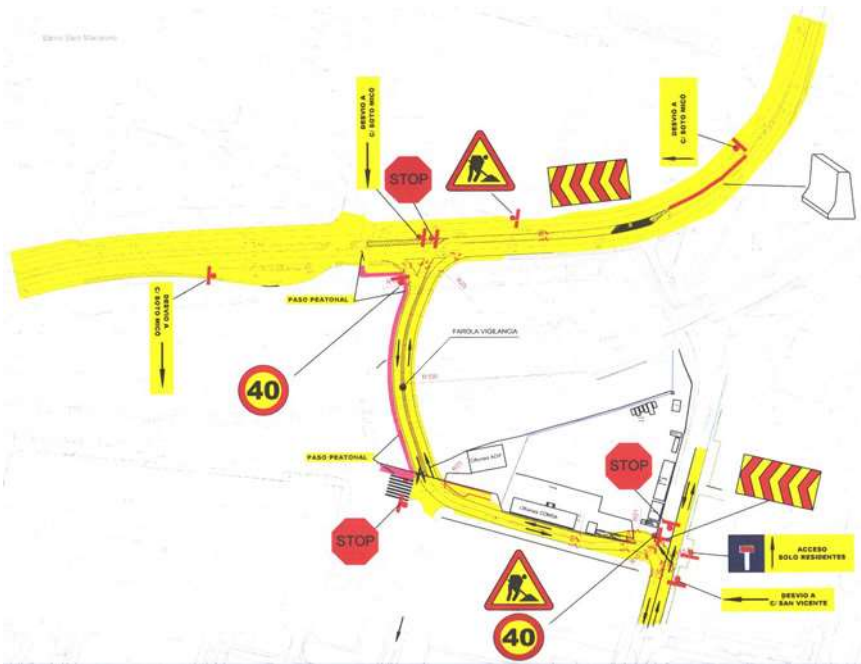
Image 3-28. Detail of diversion in construction work.
